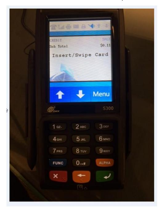
For EMV chipped cards, use the EMV reader at the bottom of the PAX S300.
